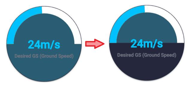
Fig. 362: Knob configuration - Full option enabled/disabled respectively
