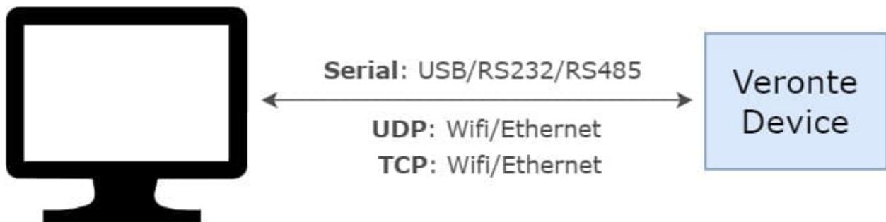
Fig. 1: PC-Veronte device connection
