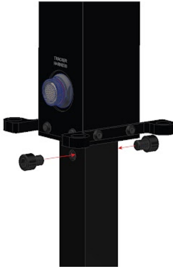
Fig. 4: Fix the T28 in to the mast
