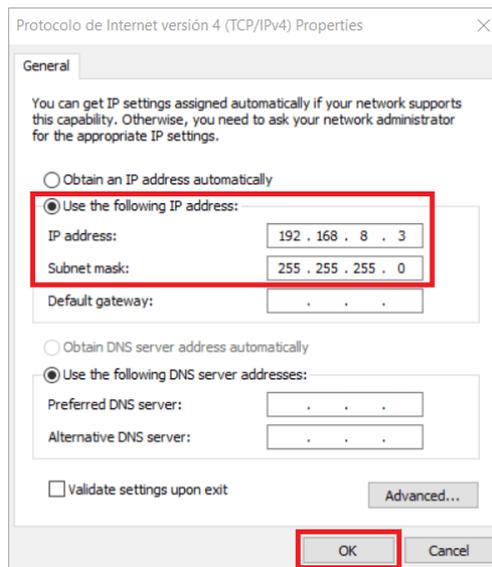
Fig. 4: IP and subnet mask configuration
