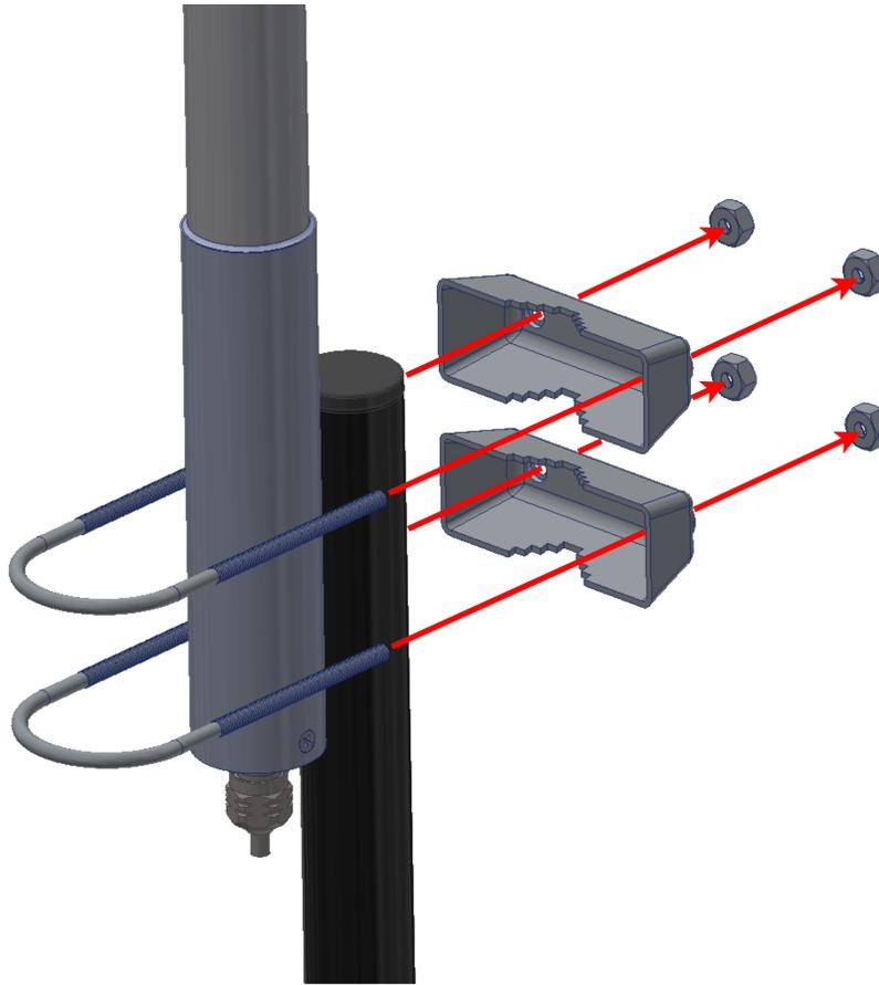
Fig. 8: Hardware SDL installation - Step 5
