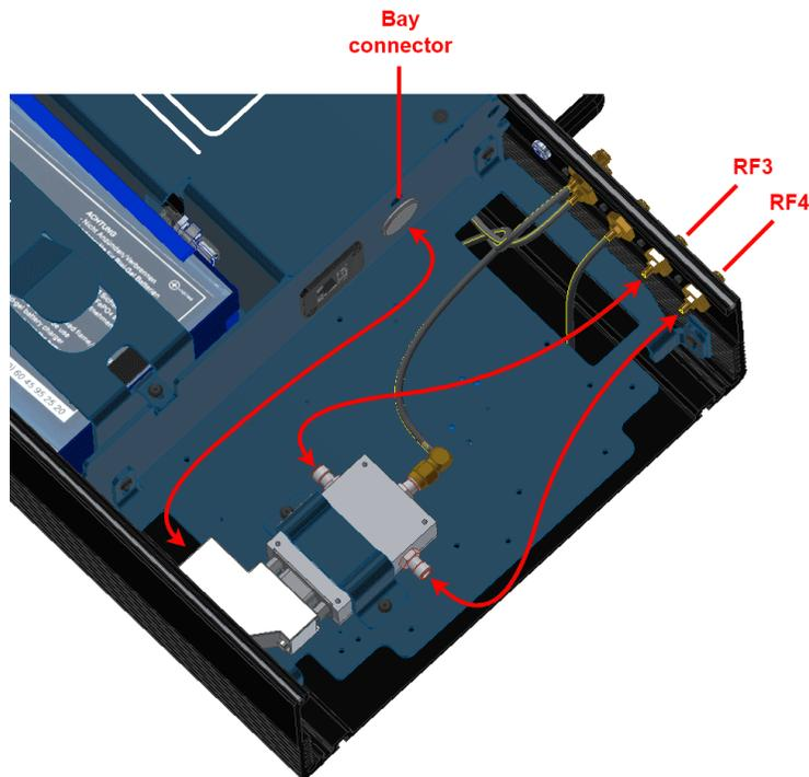
Fig. 26: Hardware Silvus installation - Step 7
