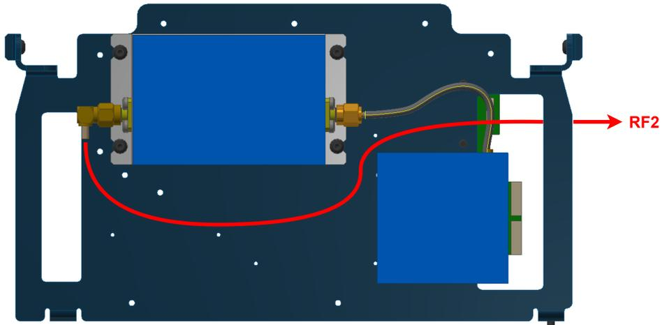
Fig. 14: Hardware DTC installation - Step 6
