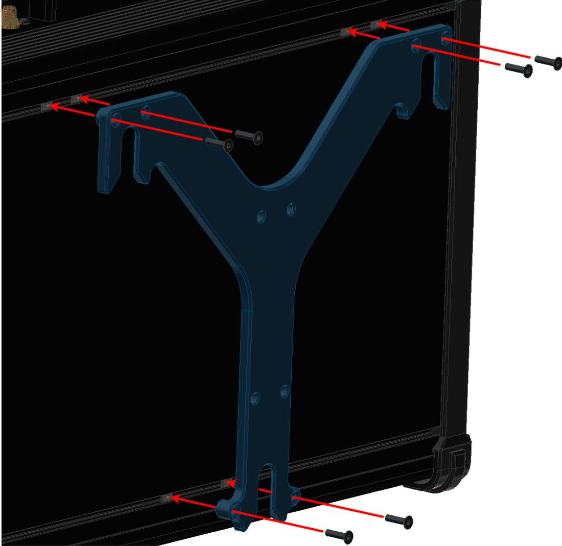
Fig. 5: Pole mount installation - Step 1
