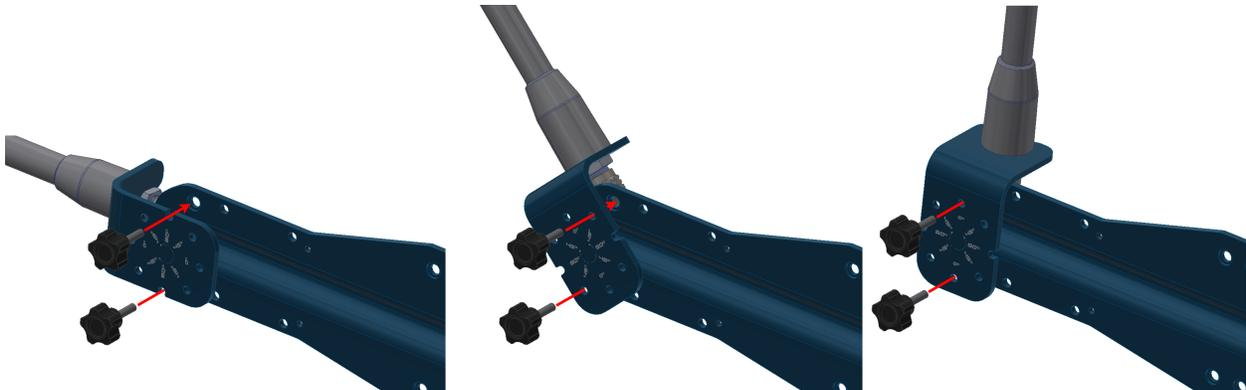
Fig. 5: Adjustable mount - Step 3
