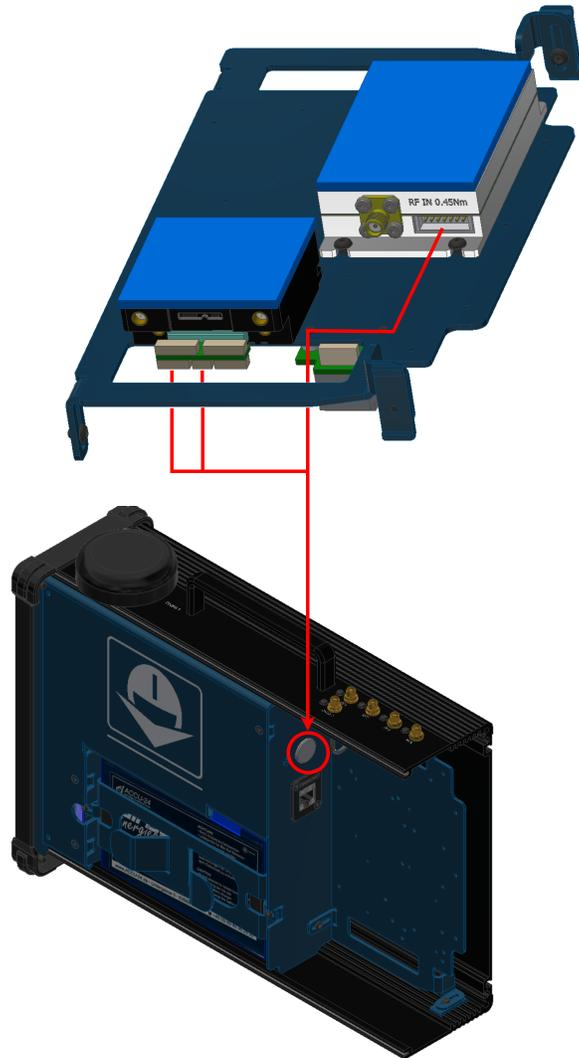
**Fig. 12: Hardware DTC installation - Step 4**
