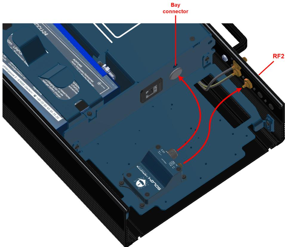
Fig. 7: Hardware SDL installation - Step 3
