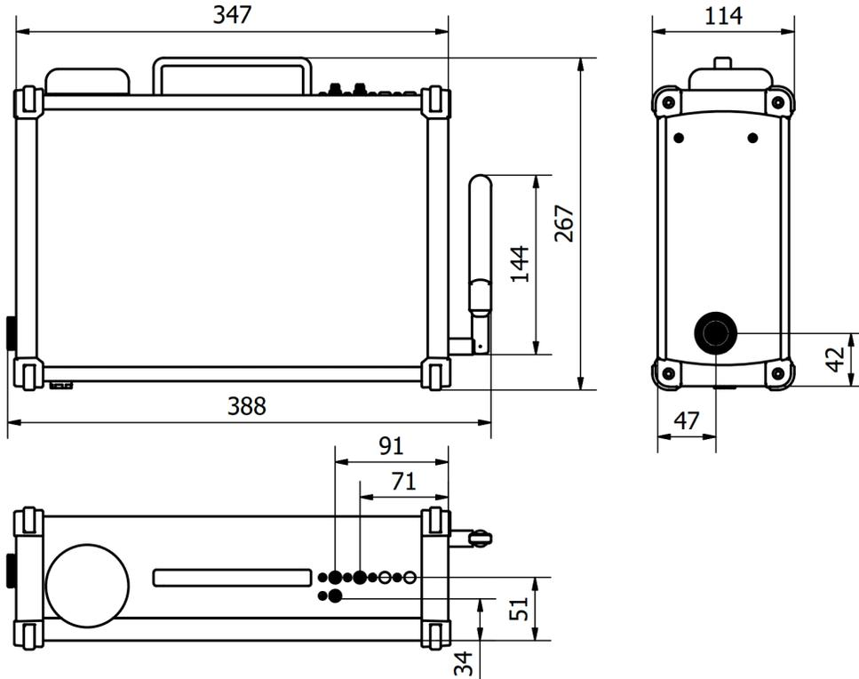
Fig. 1: Product Components - Interface dimensions
