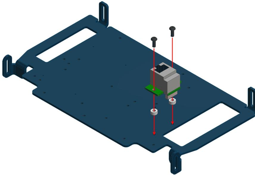
Fig. 11: **Hardware DTC installation - Step 3**
