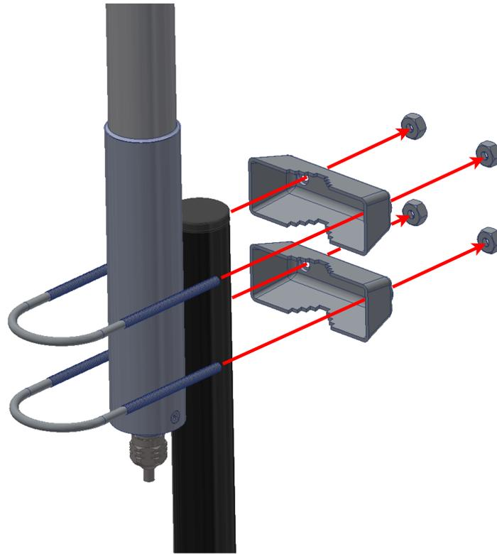
Fig. 51: Hardware amplified SDL installation - Step 9
