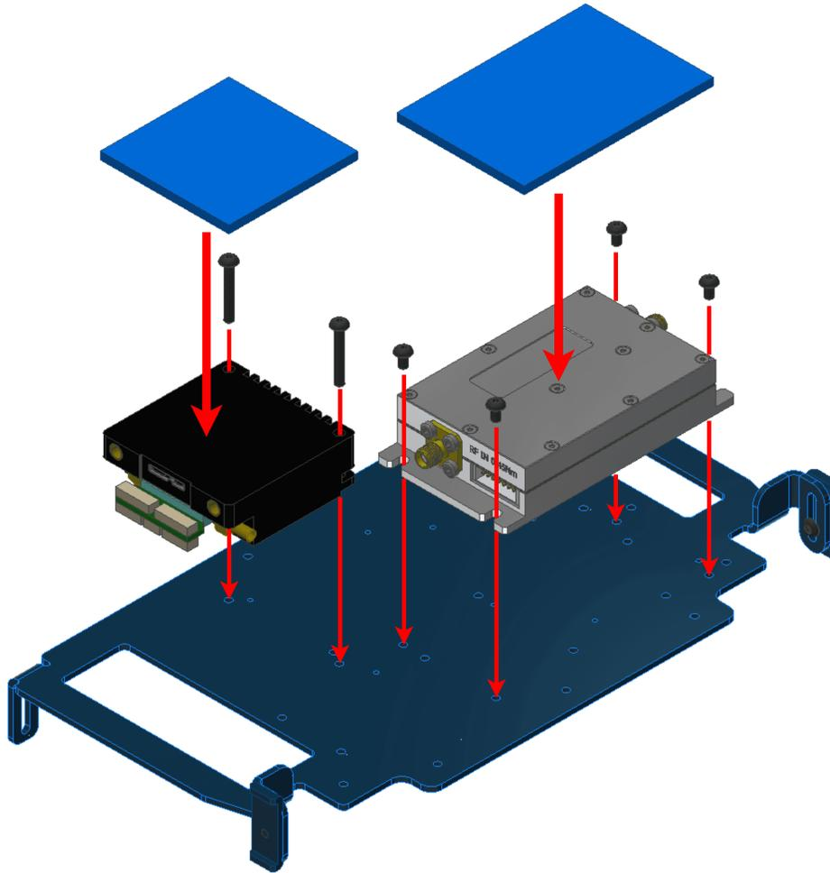
Fig. 10: Hardware DTC installation - Step 2
