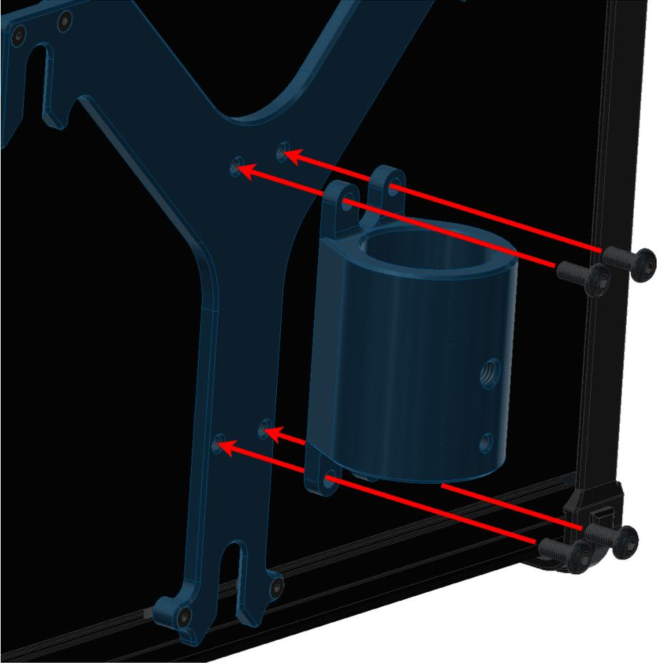
Fig. 6: Pole mount installation - Step 2
