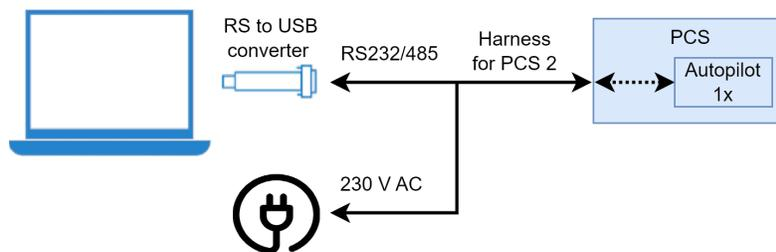
Fig. 2: Serial connection
