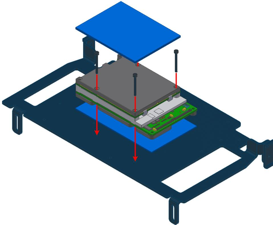
Fig. 23: **Hardware Silvus installation - Step 4**
