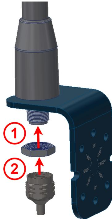
Fig. 4: Adjustable mount - Step 2
