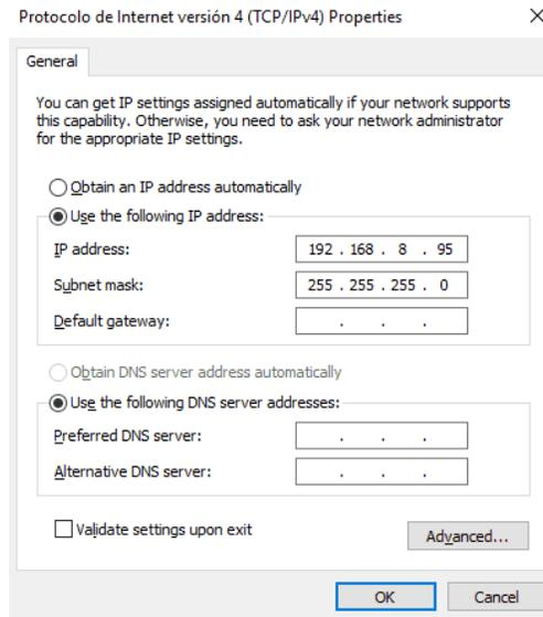
Fig. 2: Static IP Configuration example
