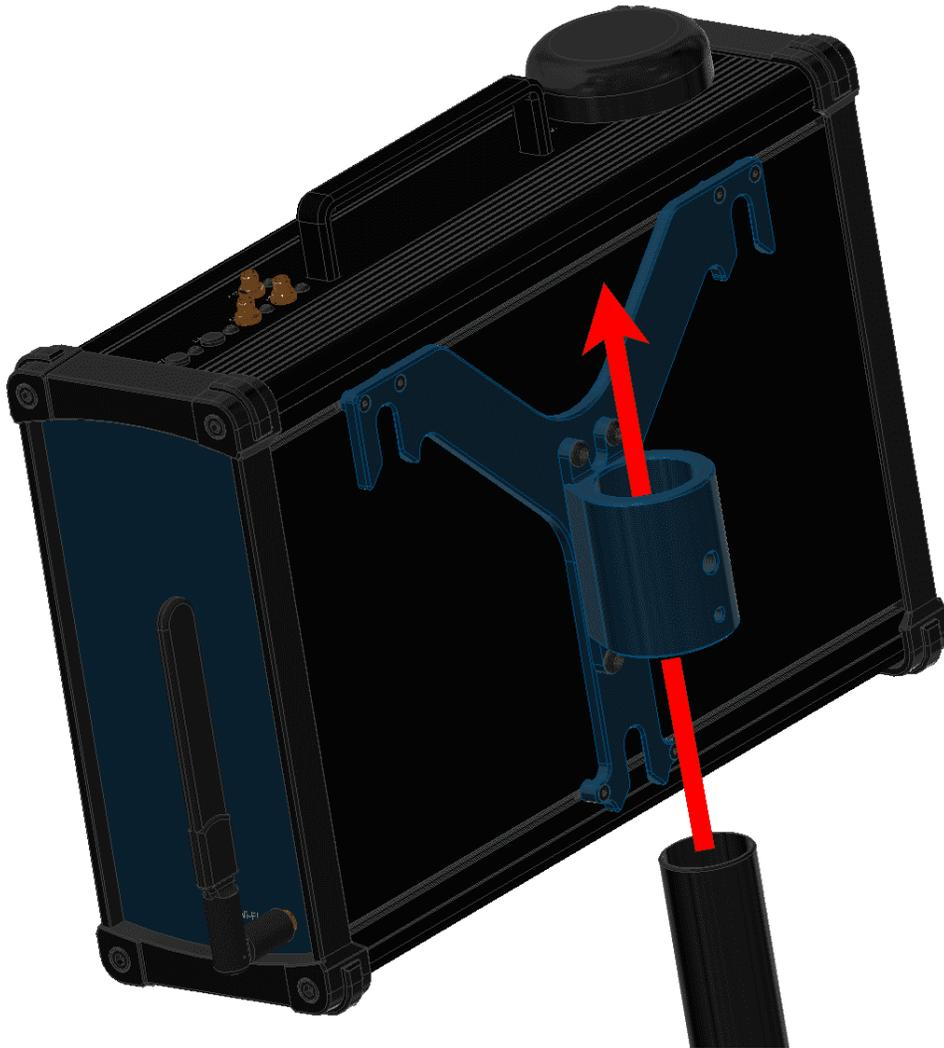
**Fig. 7: Pole mount installation - Step 3**
