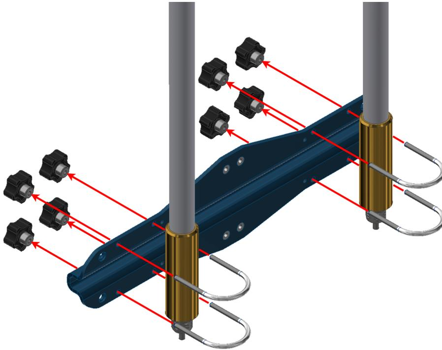
Fig. 27: Hardware Silvus installation - Step 9
