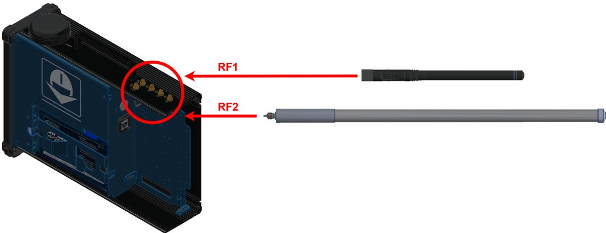
Fig. 52: Hardware amplified SDL installation - Step 10
