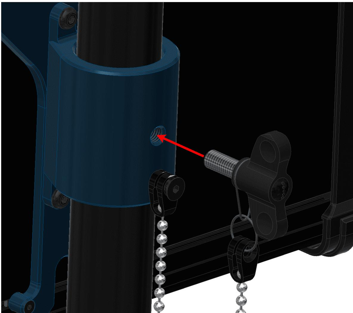
Fig. 9: Pole mount installation - Step 5
