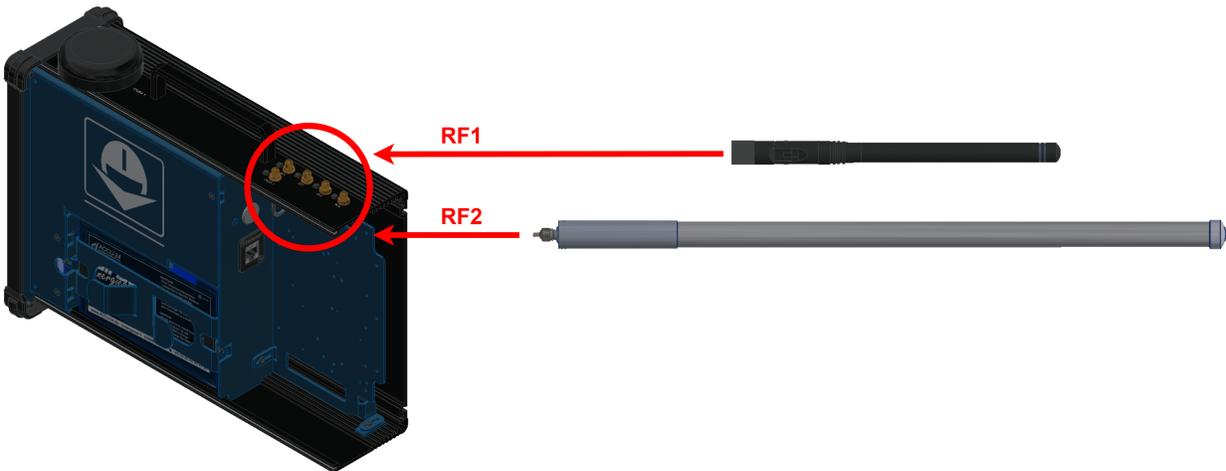
Fig. 43: MicroHard installation - Step 11
