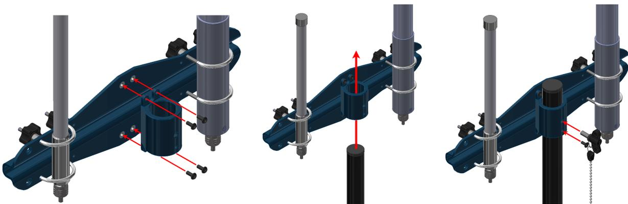
Fig. 18: Hardware DTC installation - Step 11
