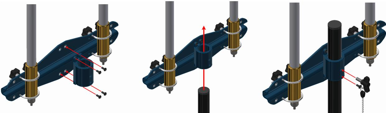
Fig. 28: Hardware Silvus installation - Step 10
