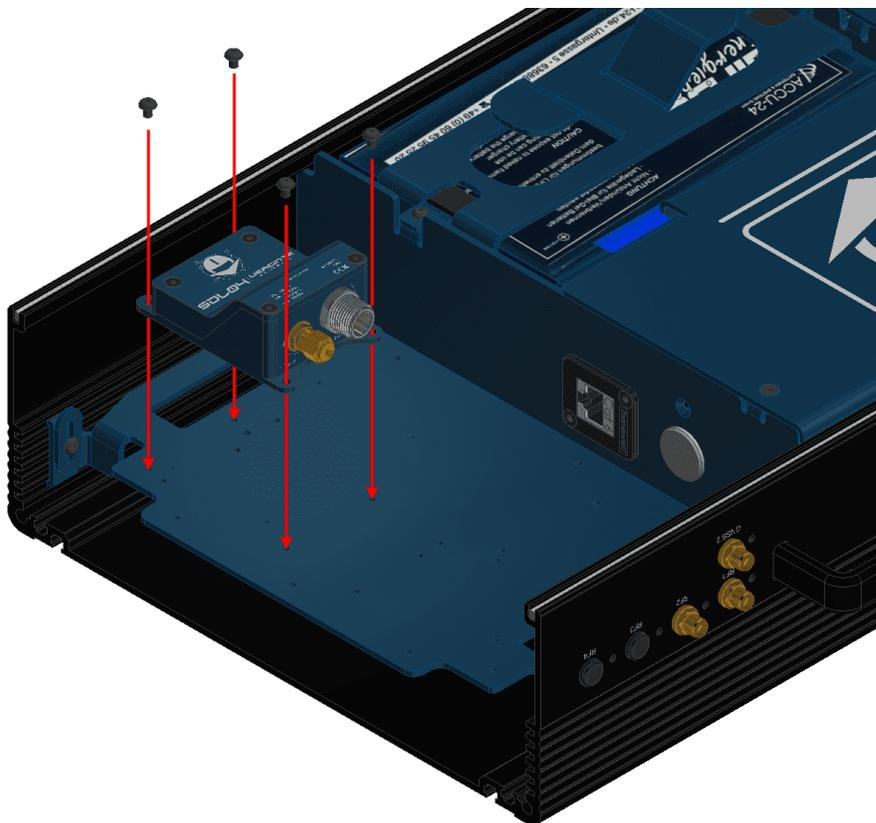
Fig. 45: **Hardware amplified SDL installation - Step 2**
