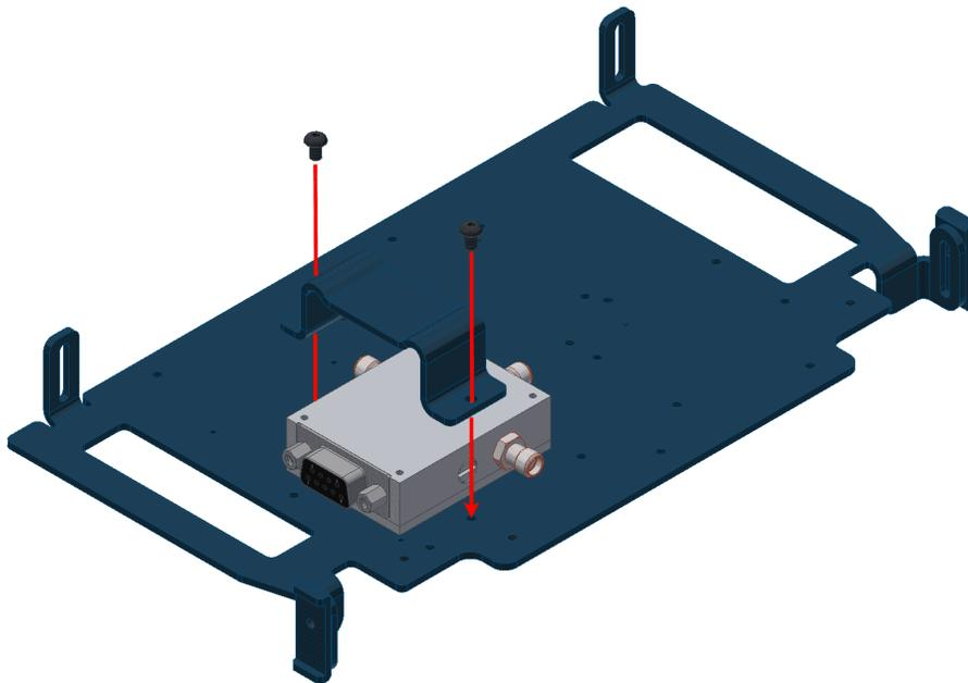
Fig. 21: Hardware Silvus installation - Step 2
