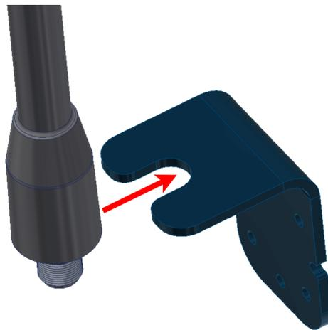
Fig. 3: Adjustable mount - Step 1
