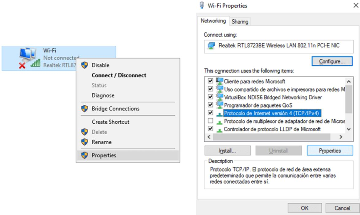
Fig. 1: How to operate - Wi-Fi/Ethernet Settings
