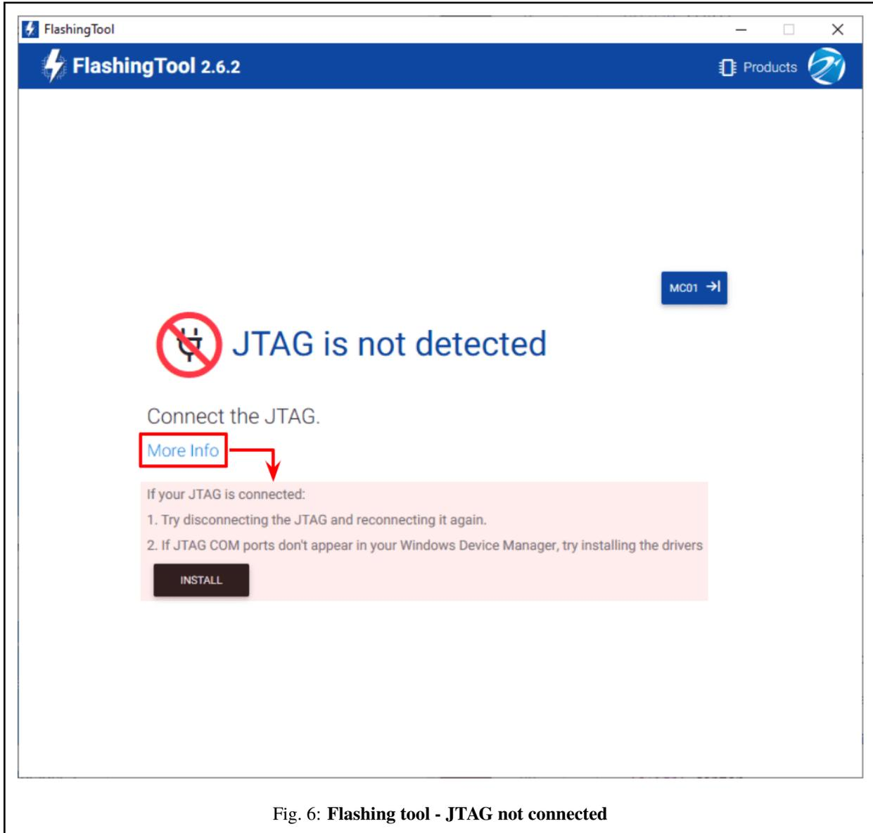
Fig. 6: Flashing tool - JTAG not connected
