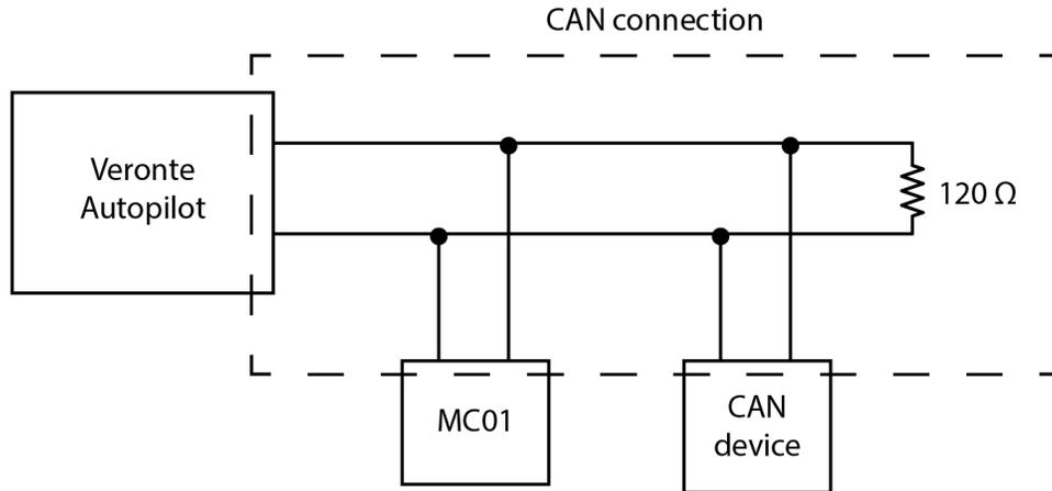
Fig. 3: CAN circuit
