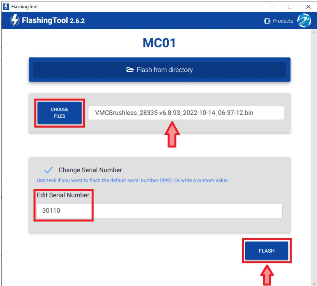
Fig. 7: Flashing tool - File and address number
