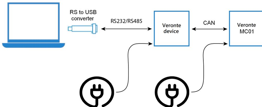
Fig. 2: Serial connection
