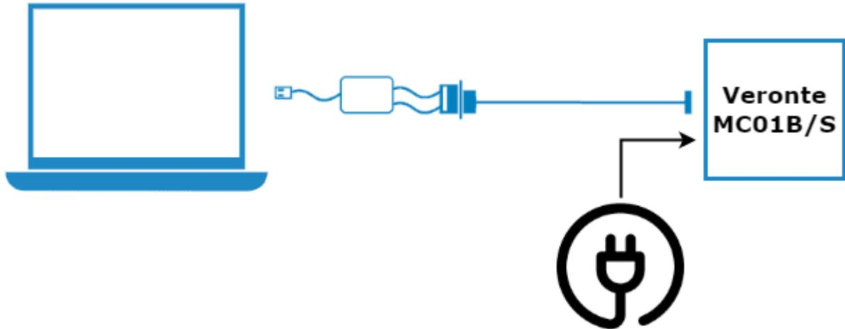
Fig. 1: PC - MC01B/S connection
