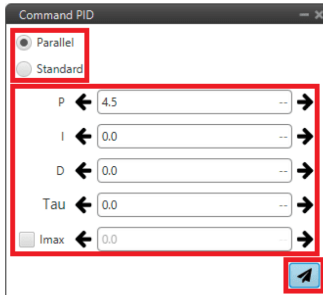
Fig. 13: Command PID panel - PID Static block
