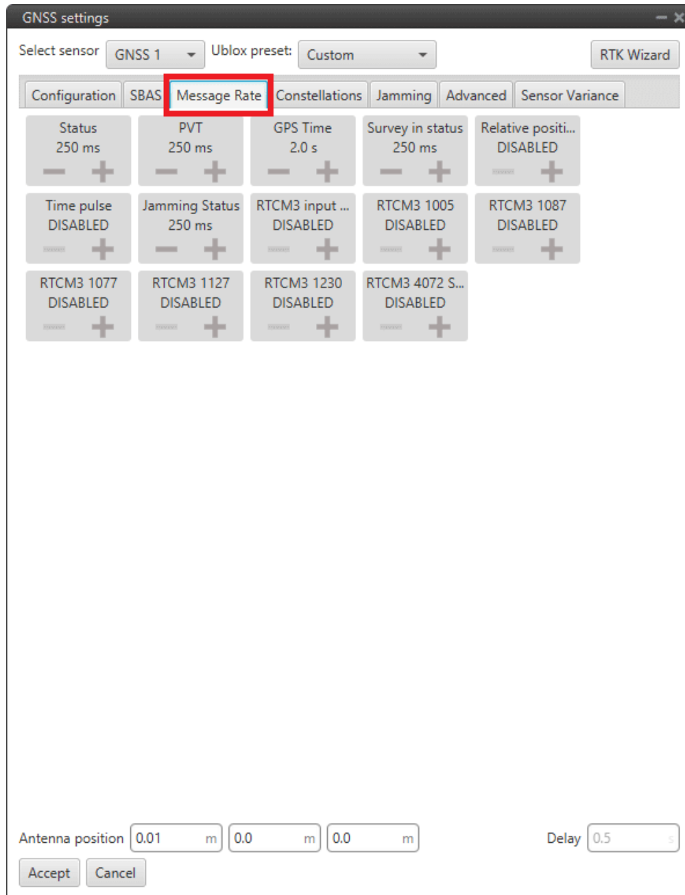
Fig. 414: GNSS 1/2 sensor block configuration - Message Rate tab
