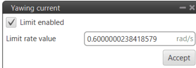
Fig. 328: Yaw current block configuration
