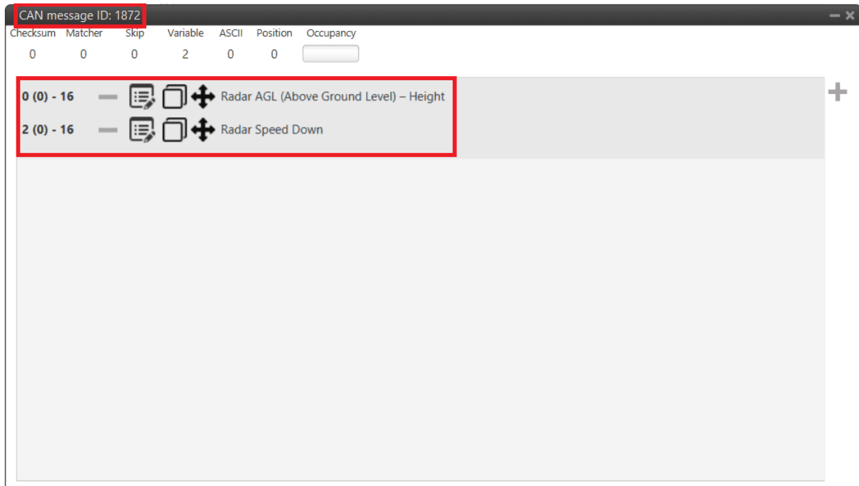
Fig. 56: Smartmicro CAN Radar - Custom message 0 configuration
