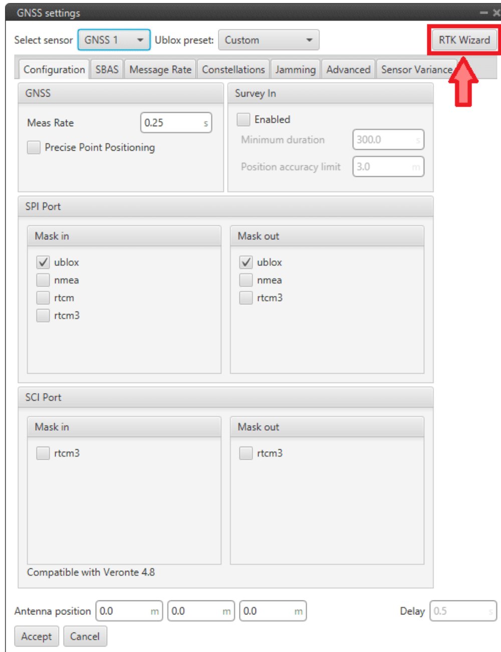
Fig. 35: RTK Configuration - GNSS block
