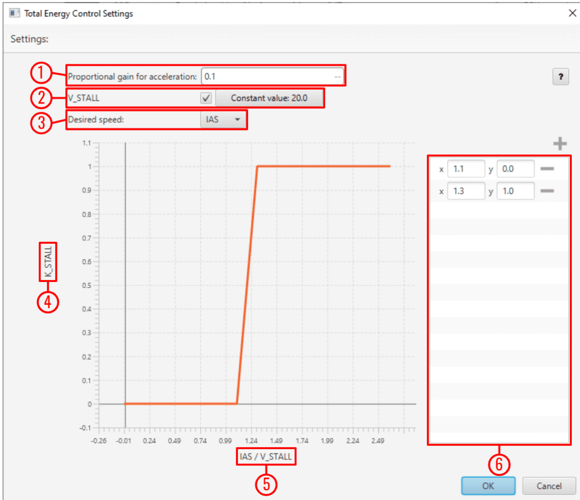
Fig. 265: Energy Control block configuration
