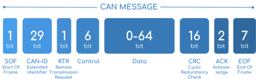
Fig. 96: CAN message structure
