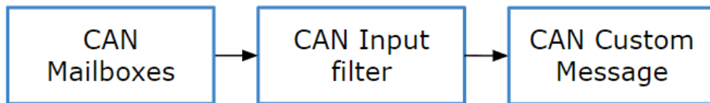
Fig. 8: CAN messages reception diagram
