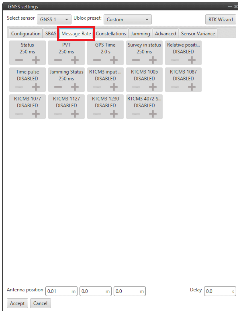
Fig. 399: GNSS 1/2 sensor block configuration - Message Rate tab
