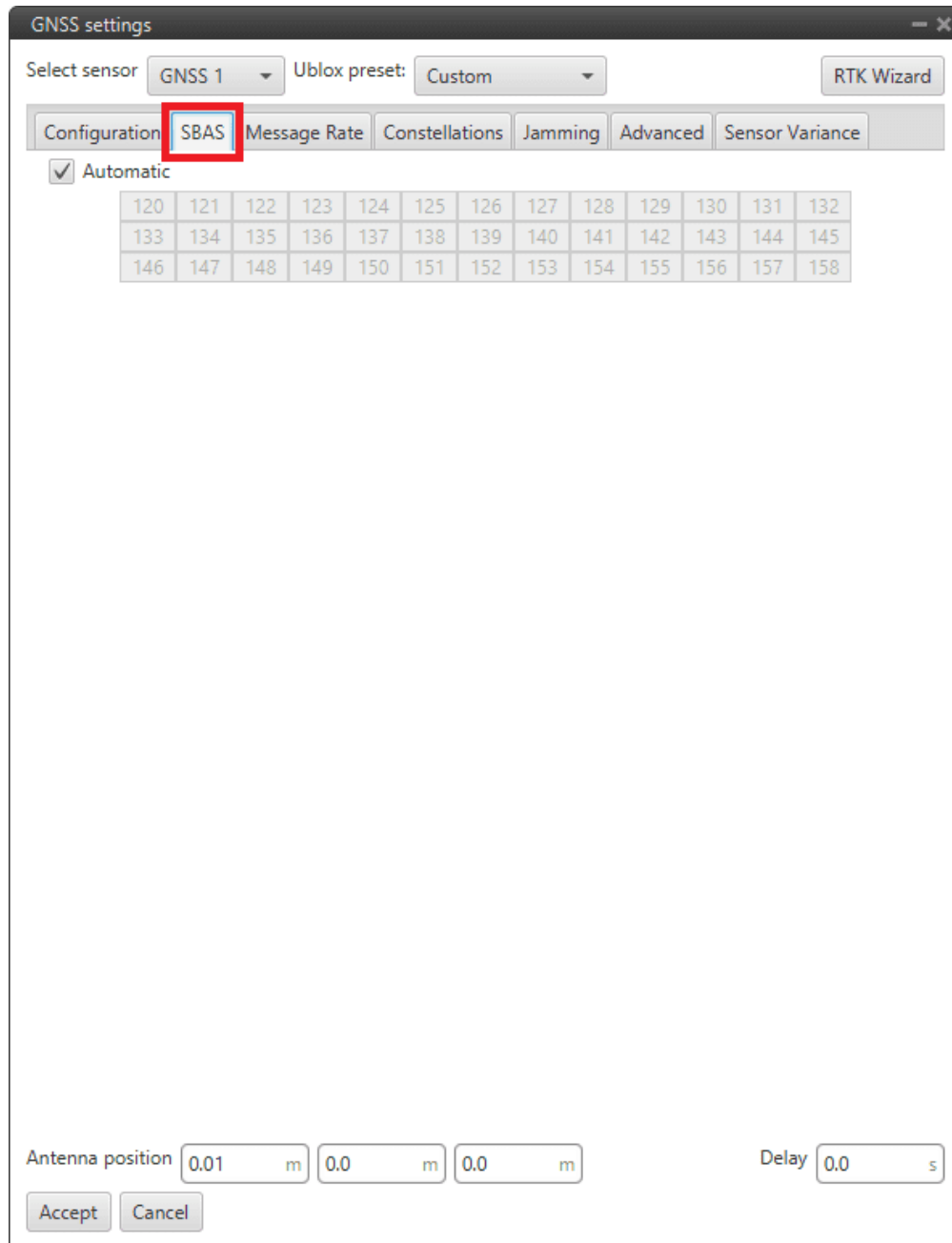
Fig. 398: GNSS 1/2 sensor block configuration - SBAS tab
