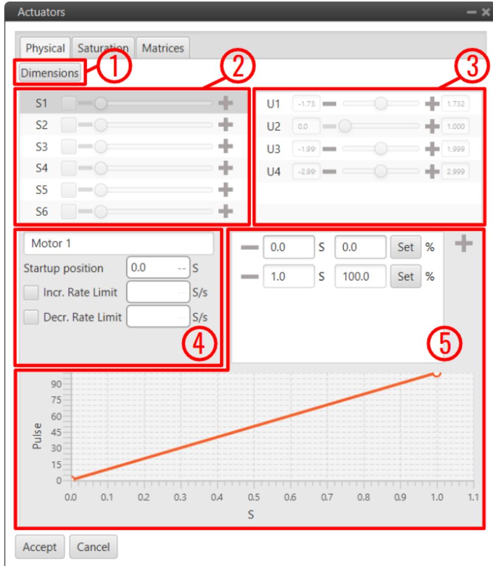
Fig. 417: Actuator block configuration - Physical
